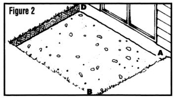
The actual excavation depth is determined by the following factors; base depth, paver thickness, sand depth, and desired finish level (see figure 1). Figure 2 shows the patio area after excavation. Locate points A, B, C & D with <sup>3</sup>/<sub>8</sub>" diam. nails. Check that AD=BC and BA=CD at the same time AC=DB. This ensures a true rectangular patio that is perpendicular to your house. A string run from A to B to C to D can serve as a visual guide.
