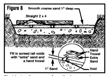
Start laying the pavers from the house out. Complete the laying process with whole pavers only. Alternate between screeding sand and laying pavers until the entire project is complete. As you lay the pavers, make sure the seams are true and square from row to row; or row to every other row, depending on the pattern you have selected.
